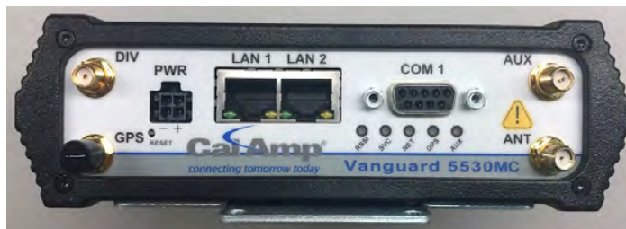
Figure 94 – Modem Front View
