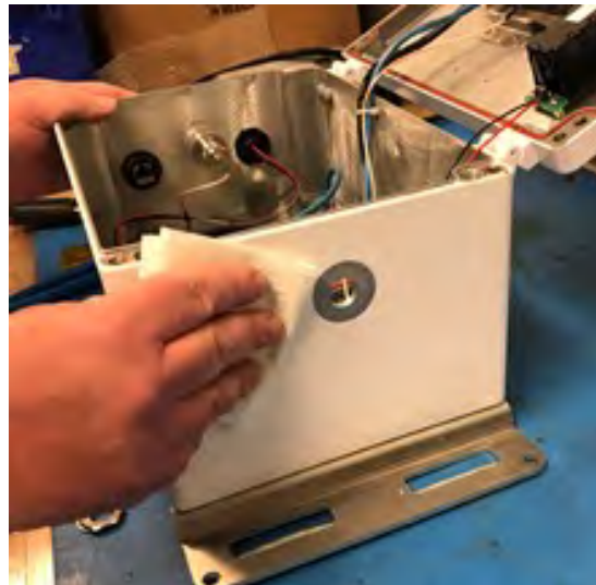
Figure 119 – Clean Antenna Mounting Area
